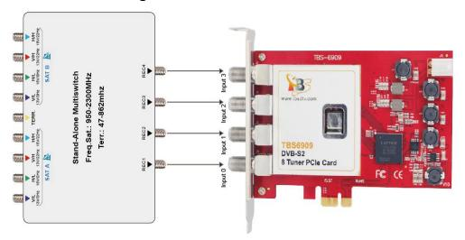
In some case multiswitch have more than one satellite input, need to choose the satellite first, then you can use this mode . It will be selected satellite by sending Diseqc command.
