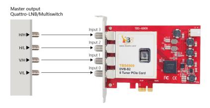
Input 0 Interface: You can only receive DVB-S/S2 TV channels from **low-frequency noise V/L TV signals.** After connecting to these TV signals through "Input 0 Interface", you can receive SD/HD TV channels from the 8 different satellite transponders simultaneously.
