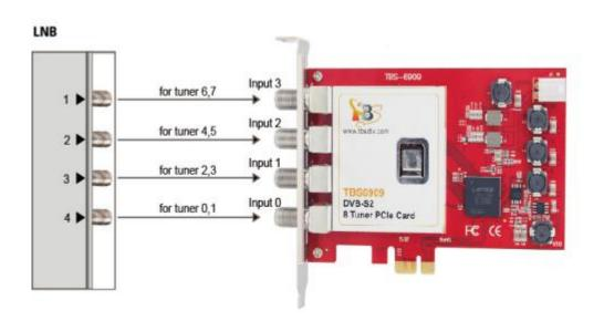
Normal mode, input0 corresponding to Tuner0 or Tuner1, can only work V or H of which a signal channel, if you want to work V Tuner0 signal channel, Tuner1 work H signal channel, is not allowed
