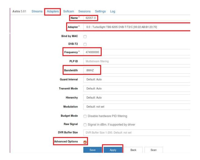
9.4 Enter into "Adapters" again. If the LNB signal indication pops up in the window, you have successfully completed the configuration. Click it and enter into the operation interface. (See screenshot below.)
