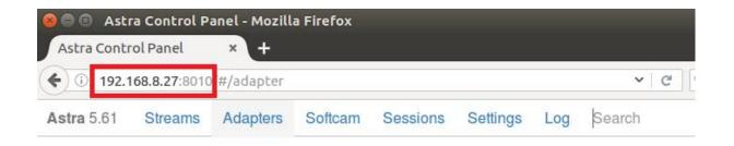
9.3 Create a new "Adapters" and then set the right satellite TV signal and frequency parameters via LNB, finally click "Apply". (See screenshot below.)
