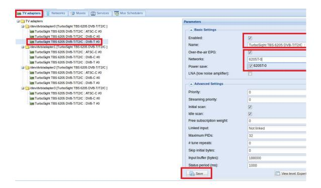
8.6 If you want to play the DVB-C signal, please perform the 8.3~8.4 step first, set up the C signal and the frequency point you need, and close the 8.5 step DVB-T signal channel. Application DVB- C signal channel, and save (as shown in Figure)
