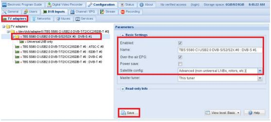
9.6 If you want to play the DVB-T signal, please perform the 9.3~9.4 step first, set up the T signal and the frequency point you need, and close the 9.5 step DVB-S signal channel. Application DVB-T signal channel, and save (as shown in Figure)
